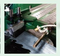
Flow control valve regulates nozzle spray.
